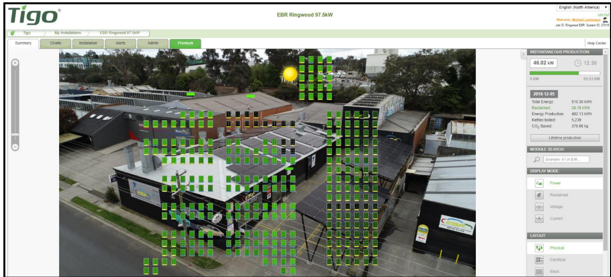
Tigo's SMART website tracks minute-by-minute module-level data via this online monitoring portal.
