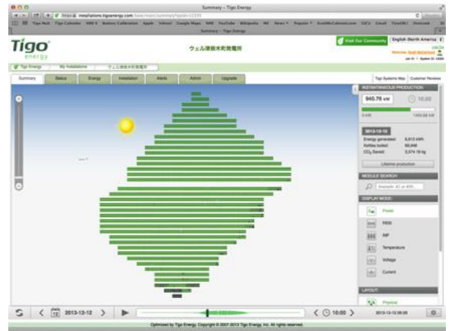
Figure 2: Installation with minor shade on the south side of the array
