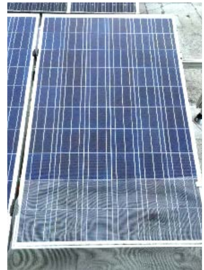
Close-up of the shaded A10 panel with a screen mesh covering 2 rows of cells.
