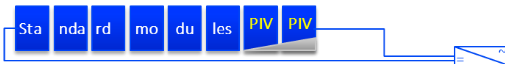
Figure 3: With Predictive IV in a single string only shaded modules require optimization
