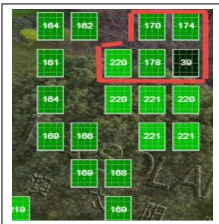
Underperforming panel doesn't impact the other panels in the same string.
